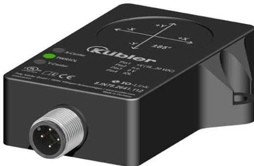
The inclinometers in the IN68 series are used to detect 2-axis inclinations in the measuring range of  $\pm 85^\circ$  or 1-axis inclinations of up to  $360^\circ$  via an acceleration measuring cell. Various parameters can be customized for individual requirements (e.g. via the PACTware software). Thanks to their high robustness, the inclinometers are also ideally suited for outdoor use.
